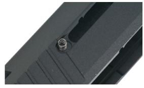
Put Part D on the slide as show in above \*\* Part D do not need glue because it infix by extractor.
