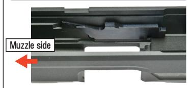
Install slide stop catch plate into the slide as show in above.
