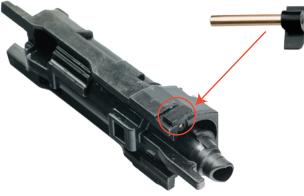
Install part B as show in above. Part B is tight because it need to fix into blowback housing. Do not file part B and use plastic hammer to put it into blowback housing.
