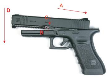
After insert from teh angle A, fit C to B and toward D.
