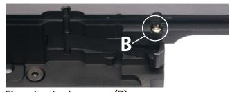
Fix extractor by screw (B). It may effect blowback function if this screw get loose. Advise you to use glue to fix screw.
