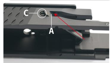
Place extractor spring (C) on hollow of slide. Insert extractor from inside of slide.
