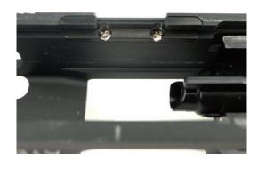
Slide Release Notch Enhaced Part (E) is screwed to fix by 2pcs of Screw (D). It is better to use screw locking glue as it may effect the performance when these screws get loosoned.
